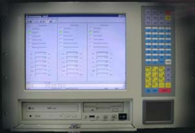
PC with software for electrode control system
